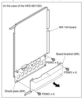
2. Install the desired board into the corresponding shield plate.
